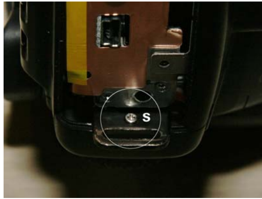
Figure 10. Removal of top cover (screw s) (camera shown upside-down)
