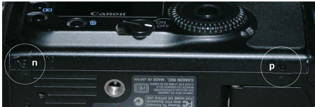
Figure 6. Removal of back cover (screws n, p)
