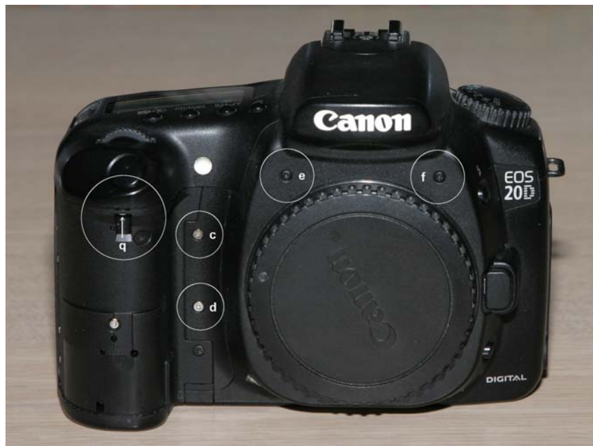
Figure 2. Removal of front cover (screws c, d, e, f); removal of top cover (screw q)
