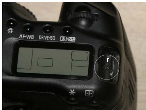
Figure 9. Removal of top cover (screw r)
