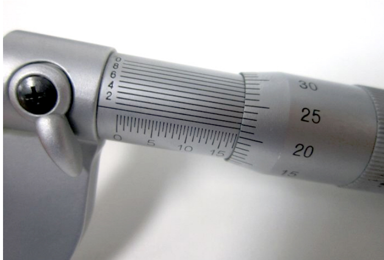
Figure 13. Vernier scale on a micrometer (millimeter)
