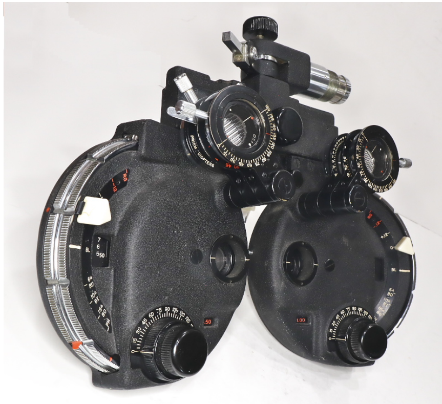
Figure 14. American Optical Model 590 Phoroptor
