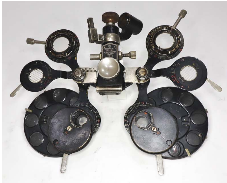
Figure 8. American Optical Wellsworth deZeng No. 588 Phoropter
