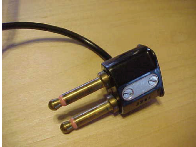
Figure 9. Headset plug (modern design)
