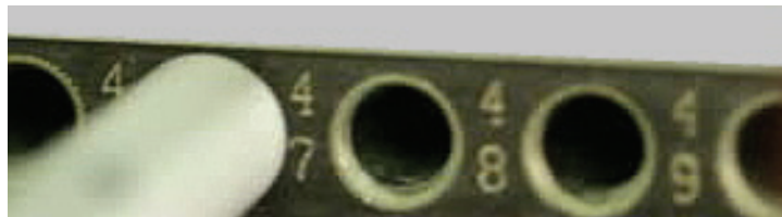
Figure 16. Multiple jack numbering
