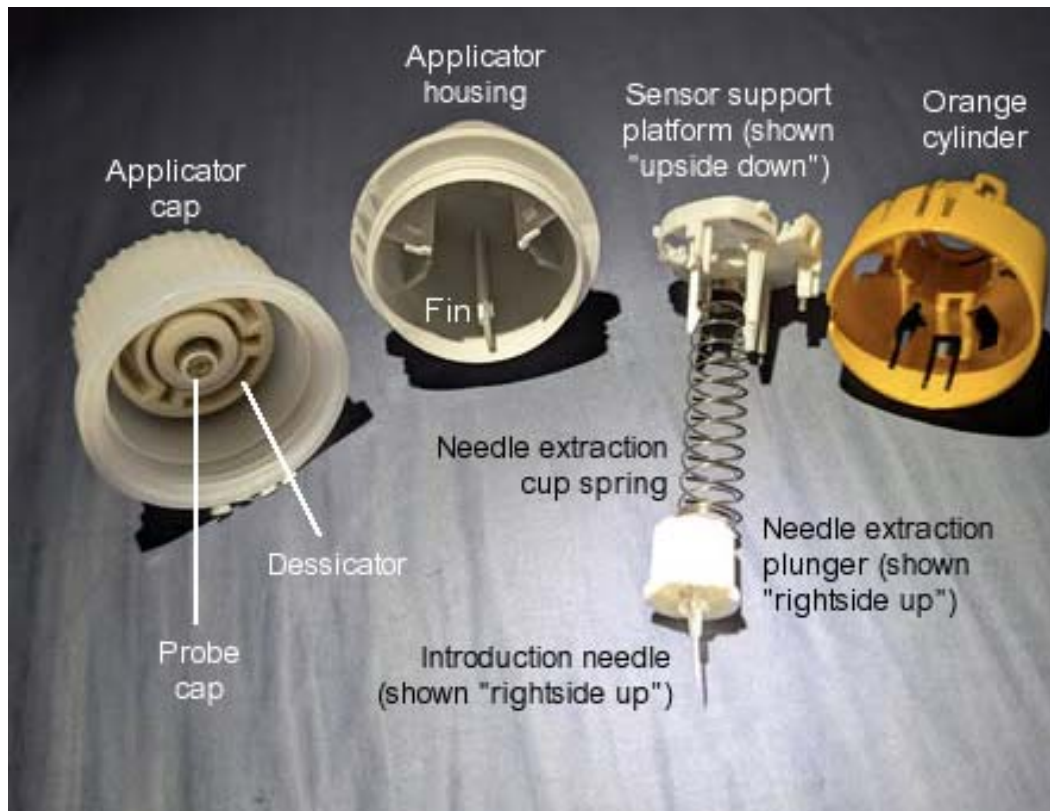
Figure 11. FreeStyle Libre 3+ applicator disassembled
