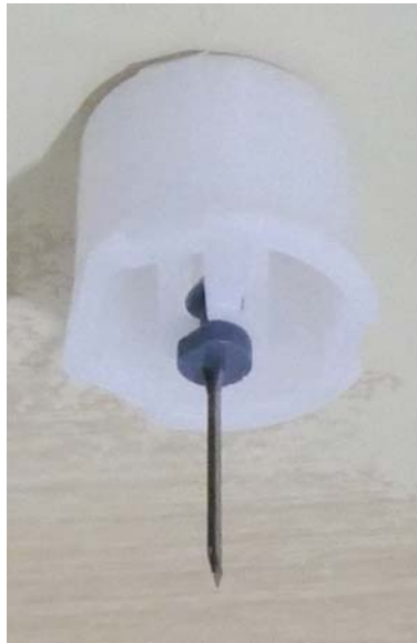
Figure 17. Introducer needle gripped by extraction plunger
