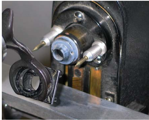
Figure 14. B&L Model 70 Vertometer—Reference axis locating pins
