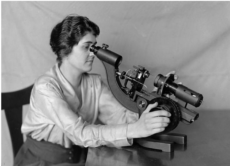
Figure 12. American Optical Wellsworth Lensometer (1920)
