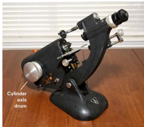
Figure 28. B&L Model 70—Cylinder axis drum
